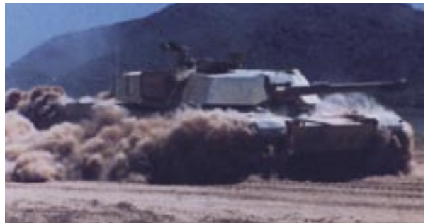
M-1 tank in desert operation. Ultra-Web nanofiber technology is currently in use on M-1 tanks extending operating time in high dust desert conditions.
