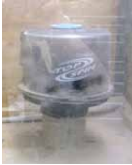
Picture of the TopSpin pre-cleaner from Donaldson design verification lab after 20 hours of ISO fine dust loading at two times zero visibility.
