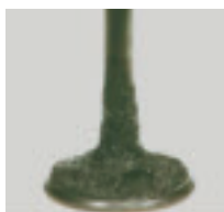
Intake valve before P.i. treatment.
