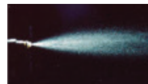
Injector spray pattern after P.i. treatment.
